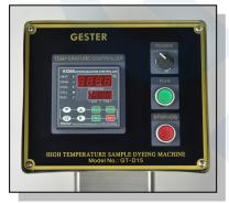
Power switch Start/Stop button Tem. Control gauge
